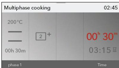
Touch the display twice to select Step 2 and Step 3. Touch the corresponding sign (step name) to confirm or delete a step.
